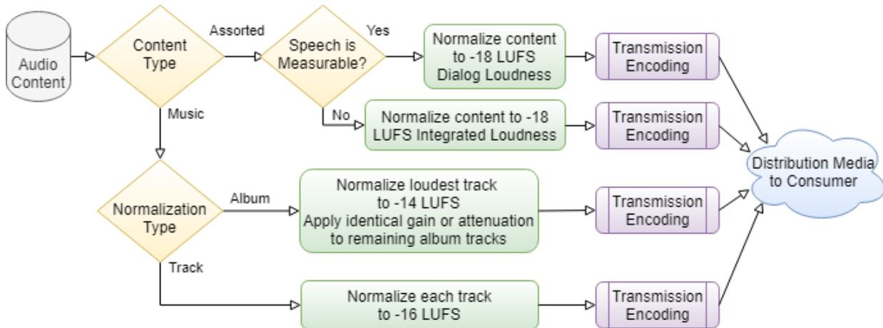
Figure 2 – Example of content delivery workflow, assorted content
