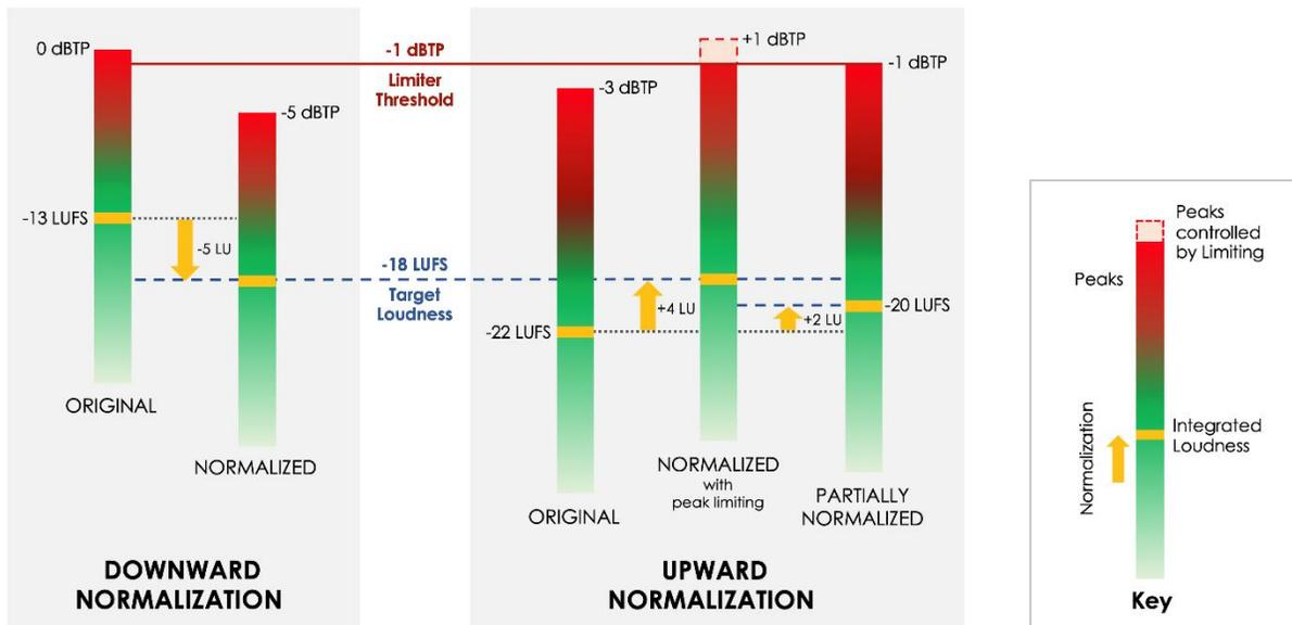
Figure 1 - Processes for Downward and Upward Loudness Normalization
