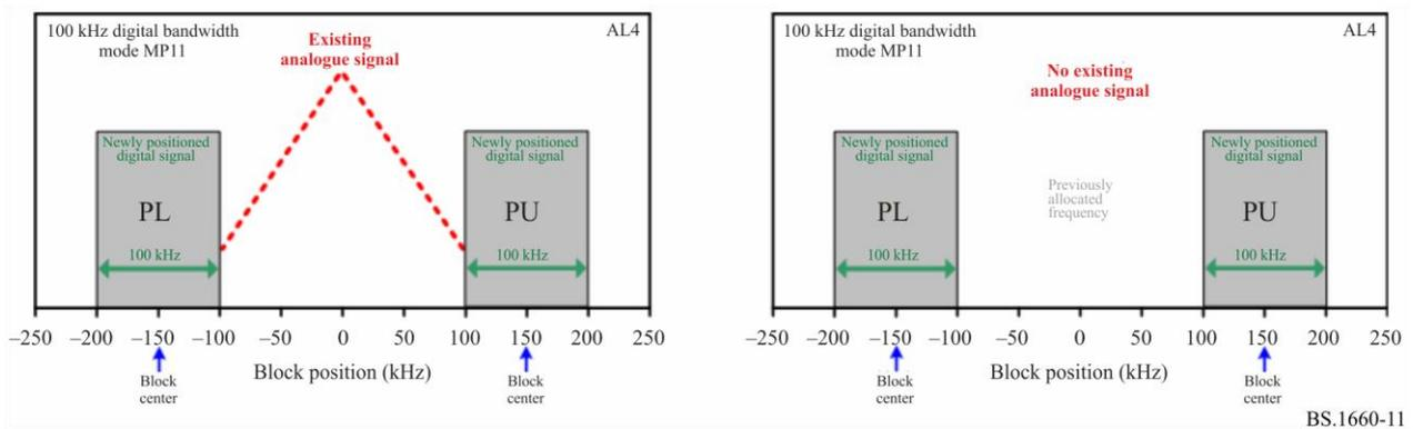
NOTE – PL and PU are used for indicating lower positioning and upper positioning (respectively) of the digital block. The indication is for convenience only, and does not suggest an actual difference in the signal.
