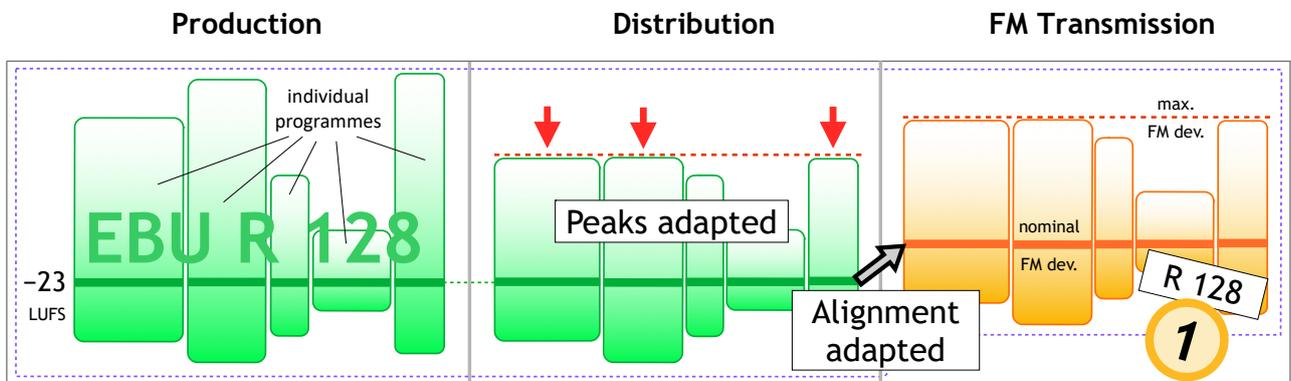
Levelling Scheme for a Radio station using R 128 compliant loudness normalisation at  $-23$  LUFS in Production and Distribution with adapted alignment for FM (R 128 **1**). Mild peak limiting and/or dynamics processing is performed where needed (see the red arrows)
