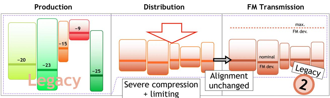
Levelling Scheme for a Radio station using no normalisation in production with legacy processing and alignment for FM. The resulting average loudness is the same as in Figure 1. Severe peak limiting and compression lead to a less dynamic, more squashed sound (Legacy **2**).
