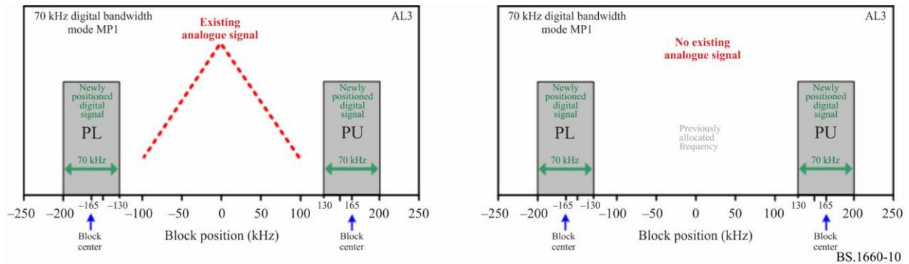
NOTE – PL and PU are used for indicating lower positioning and upper positioning (respectively) of the digital block. The indication is for convenience only, and does not suggest an actual difference in the signal.
