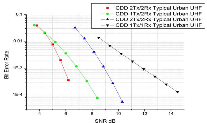
Figure 1 BER vs. SNR with Cyclic Delay Diversity
